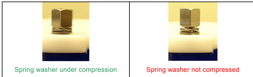
Figure 11. M6 Standoff Bolt on Electronic Housing Cover Plate
